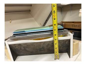
After firing, the skim glass left on the stainless bars will "spit" off the stainless so you will need to vacuum after each firing. It does not damage the glass bar or the kiln as it happens at about 500 on the cool down. To reuse the flow strip, I just
