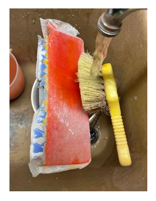
Here is the resulting fired bar in my sink. There will always be spikes on the top of the bar so watch out! Dump it out of the former and take it to a sink and scrub it with a green scrubby or brush until all of the fiber is removed. If you have a sandblaster, when most of the fiber is off, you can finish it up by blasting. If you have a grinder grind off the sharp spikes. The cleaner you get before slicing, the better.
