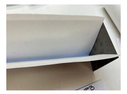
3. Next Cut 4- 4 1/2" by 5 1/2" out of the 1 mm fiber.....Place a dot at the center point of one of the 4" sides and draw a 45% angle to both corners and cut it out. Cut outside the marker line.These should be slightly larger than the end of the pattern bar former so that when you push them into place they overlap the other fiber. I trim the tip off as in the picture.
