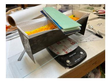
In my kiln on this firing, I put some 1/2" old fiber board on the brick with no shelf and loaded it. If you put it right on brick be sure it is kiln washed or put thinfire under it as a precaution, (especially on your first couple of bars) Notice the kiln stilts holding the fiber board in place.
