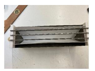
Trim the top edge of the triangle fiber liners where the flow bars will be.
