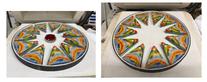
It worked perfectly although I was unhappy with the red center so in the final firing I covered it. These slices have 5- 3 mm clear under each bar. I fired these fast! 500/1520 hold 2 hrs 9999 to 950 for 2 hrs 100/600/off
