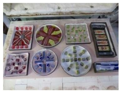
Kiln getting prepared for loading. Fresh Bullseye kiln wash 3 layers liberally applied.....next picture 1/8" fiber paper on the insides of all the forms. Make to put a scrap of thin fire behind the joint and the fiber is pressed against the shelf. I could add more forms and pack it tighter but it is alot of glass and I like to give it a little room!
