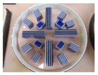
The important thing to remember in this technique is to put in enough glass by weight that it will flow to fill your ring. To do that we are constructing a chart with our rings that will make it easy for you. These will be apx 3/8" to 1/2" thick. When you have perfect
