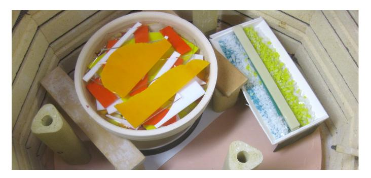
Here is a load with a Bubble Pot Melt Pot and a Triangle Pattern Bar in the same load. They play well together at these temps. when using triangle bars at high temeratures be sure to line the entire bar with 1.8" fiber paper sealing well at the ends. This pot mix resulted in the piece at the top of the page.
