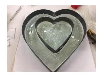
Be sure when lining any stainless steel form that the ends of the fiber are cut carefully so that the 2 ends will meet flush. This joint should have a 1" tall scrap of thin fire behind it. This is a bit of insurance. The fiber can shrink and by doing this the stainless will not be exposed. I do not prefire, spray or kiln wash the stainless. It is just not necessary.
