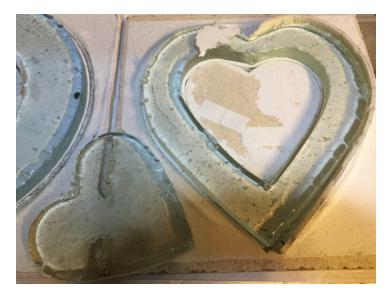
The small heart I would cold work and then add any color or whatever and fire it again out of the stainless. I did this one really crazy just for this test. The clear was thick so I ended up with about a 7" heart firing it to 1420. After firing it to full fuse with the color I cold worked it and into a fire polish.
