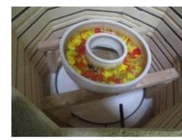
Next step: \*Use 1/8" fiberpaper lining the ring. After you have the fiber paper cut perfectly.....if you have some Zyp .....take your strip of 1/8" fiber paper outdoors, hold it on one end and spray it with Zyp from top to bottom on the smooth side that will touch the glass. This will significantly reduce the 'spiky needles' from glass dragging on your fiber paper and thereby
